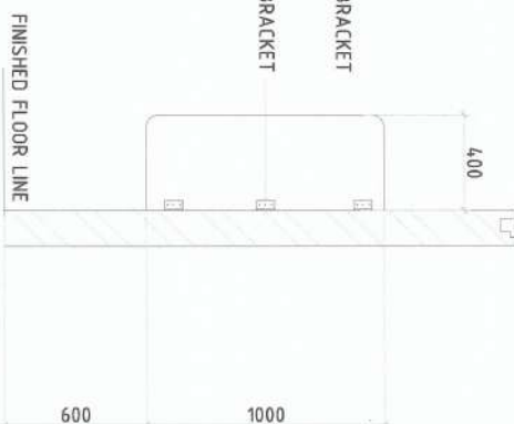
MODULAR PARTITION DETAIL (FOR URINAL & CUBICLE) SCALE 1:50
